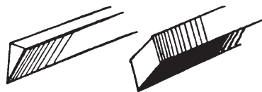
Pointed burin for copper engraving
