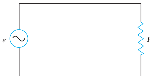
FIGURE 7.1 AC voltage applied to a resistor.
