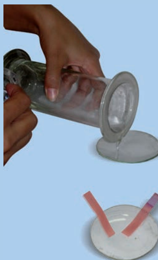
Fig. 4.4 (b) : Testing of solution with litmus papers
