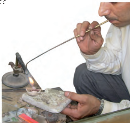
Fig. 6.14 : Goldsmith blowing through a metallic pipe
